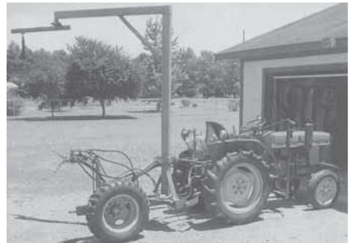
**Remote-operated rig is used to trim Christmas trees. Steering is controlled by pivoting the whole control unit, which is connected to the steering linkage.**
