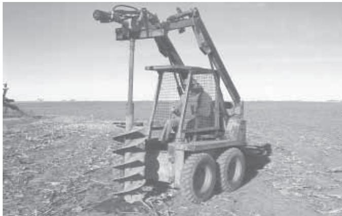
**Marshall Litchfield used a Kinze grain auger to make a big "earth auger" that digs 18-in. dia. holes as deep as 9 ft. Auger flighting was doubled up on shaft.**
