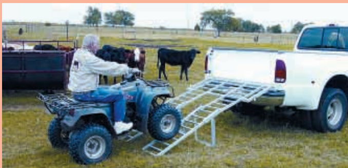
Safeload Tailgate attaches like a pickup tailgate. When fully extended the ramp is 85 in. long and 49 in. wide. Angle iron brace folds out under middle for added support.
