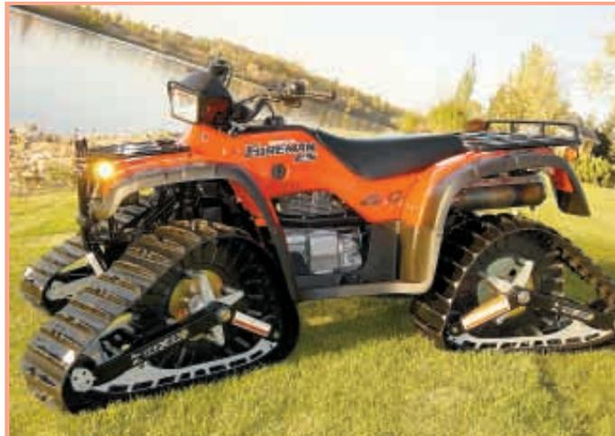
TraXion kit converts ATV’s to tracks for year round use. Once kit is installed, you can switch from tracks to wheels in about 15 minutes.
