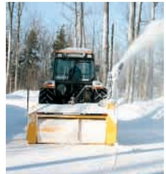
By rotating shield to cover back of auger, operator can blow snow while driving forward.
