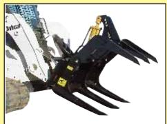
Also available from Sidney Manufacturing is the Gorilla Grapple, a powerful grapple designed to fit most skid steers. Manufactured from high tensile 1-in. thick steel, the grapple can handle debris, large trees, big hay bales, salvage yard scrap, and even crushed concrete slabs. "Designed by grapple customers to handle anything a skid steer can handle."
