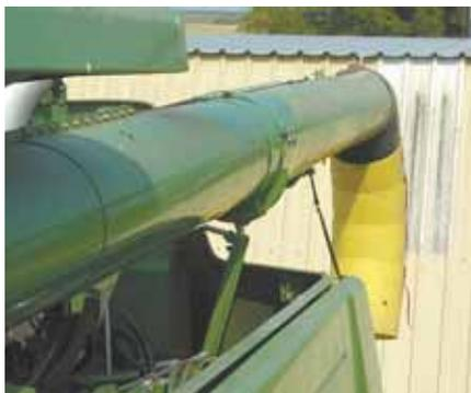
To stabilize the unloading auger on his Deere 9650 STS combine, Roger Gutschmidt bolted a home-made bracket to the combine's frame.
