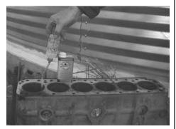
Applicator dispenses chemical around cylinder wall. It can also be squirted in through spark plug or nozzle openings.
