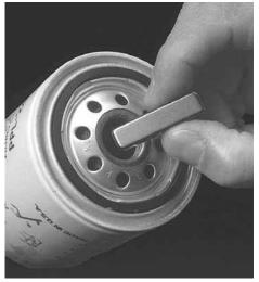
Magnet catches particles too small for an oil filter to stop. It's designed to be dropped into the center hole of any spin-on oil filter with a metal core.
