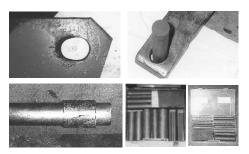
Elongated holes (top left) can be repaired by simply inserting a Repair Tech rod and welding around it (top right). Cracked bushings (lower left) can be welded right on a rod. Two kits are available (below right).
