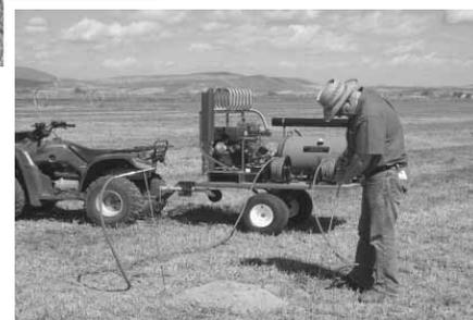
The wand is used to fill rodent burrows with pressurized carbon monoxide.
