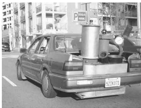
**Wood gas generator turns wood and other biomass into gas to fuel cars, trucks, stoves and furnaces. Car shown above is running on syngas. A completely assembled unit is shown at right.**
