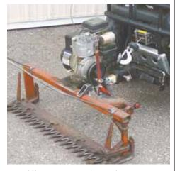
Modified walk-behind sickle mower mounts on front hitch.
