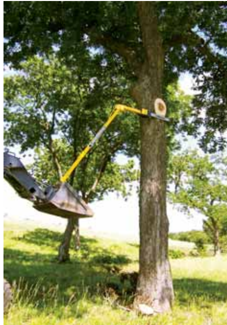
Tree trimmer has an 8-ft. mast and mounts directly to receiver on front-end loader.
