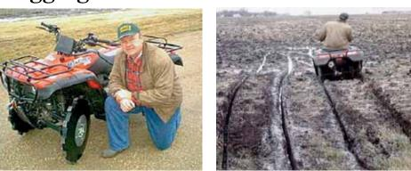
Wheels make a 3 to 5-in. deep trench in muddy ground. Deeper trenches can be made by making repeated passes in the same tracks. Works great for draining water away from flooded fields.
