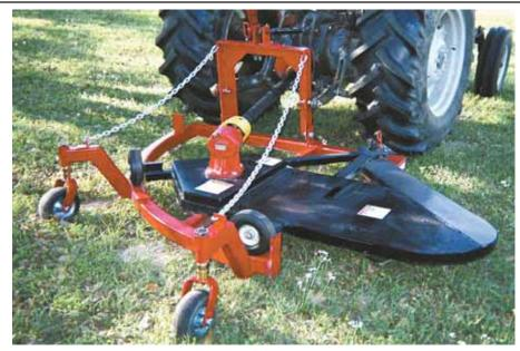
Fence Mower mows under fence lines and maneuvers around fence posts.
