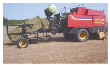
Caster wheel-mounted bale stacker is designed to always trail in line with baler's bale
