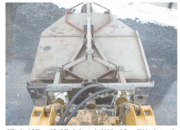
"I like the visibility and flexibility it gives me in thick brush," says Shirk, who turned a zero-turn rough-cut mower into a big mower by mounting it on skid steer loader arms.
