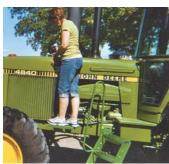
Non-slip fuel and access steps make it safer to work around Deere 20, 30, 40, 50, and 60 series tractors.
