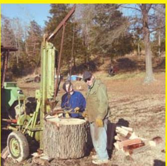
My home-built log splitter has a lift arm attached to the top. A 2-point grab hook lifts wood up to be split. The hook releases as the wood drops onto the splitter. The splitter can handle wood pieces that weigh up to 300 lbs. and measure 24 in. in diameter. (*Larry Zenz, HC 60, Box 154, Parks, Ark. 72950; ph 479 577-2677; zie7@ipa.net*)
