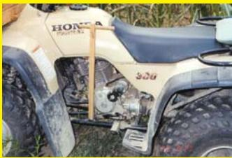
My wife is the primary driver on our manually-operated Honda 300 ATV. Because of arthritis in her foot, she was unable to engage the shift pedal. I made a hand-operated lever by cutting a slit in the bottom of a 2 by 1-in. piece of oak. I used a hose clamp inserted through the slit to fasten it to the shift pedal. At the top of the oak piece, I drilled a hole to insert a dowel for a handle. (*Bernard Paumier, 10335 Heimberger Rd., Baltimore, Ohio 43105 ph 740 862-8262*)
