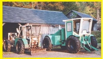
Back in 1991 FARM SHOW published a story on my front-mount 4-WD articulated tractor, which positions the operator right up front for perfect visibility. I still have the tractor, which is powered by a Ford 140 cu. in. 4-cyl. water-cooled gas engine, with both driver and engine protected by a wire brush cage. The 58 hp tractor is equipped with front or rear pto, front and rear 3-pt. hitch, foot-controlled hydrostatic 4-WD, center articulation and oscillation, and four 11.2 by 24 ag tread tires.
