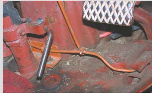
**Horizontal rod with big bend in it runs across floor from steering column toward brake latch. Another rod extends vertically up toward steering wheel.**
