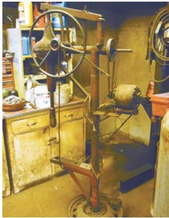
wheel rim the unit stands on. To start the press, I step on an old-fashioned starter button located on the wheel rim.
