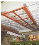
ment, where they were always in the way. "The racks were pretty easy to build and are made of 2 1/2-in. formed angle and miscellaneous flat straps for bracing. I made each of them in less than 1 hr. and they were inexpensive, as far as the materials I used. I painted them, and then bolted them to the ceiling of my loft area in my shop. They're low enough that I can just
