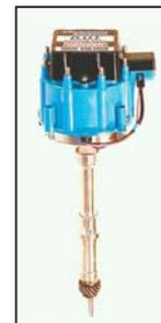
"The Dyna-Module and D.U.I. Coil work in tandem to produce a longer duration spark, allowing you to open up your plug gaps to .055. This burns your fuel more completely. The D.U.I. performs without a ballast resistor. Full voltage goes straight to your combustion chamber. Performance Distributors calibrates every D.U.I. on a distributor machine with a very accurate timing curve throughout the entire rpm range. This ensures instant throttle response when you "step on it."
