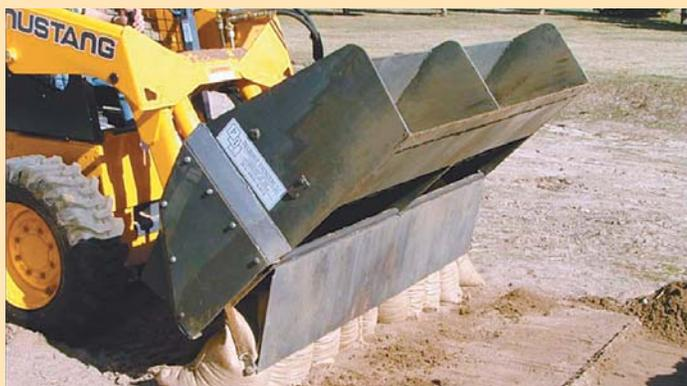
Sandbagger attached to skid loader is designed to fill 12 bags at a time. It's basically a large scoop with 12 sets of bag holders on back.
