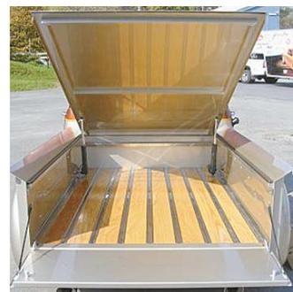
Pro's Pick builds classic pickup beds for 1930 to 1980 trucks. Photo shows oak floor filled with smooth stainless steel strips.
