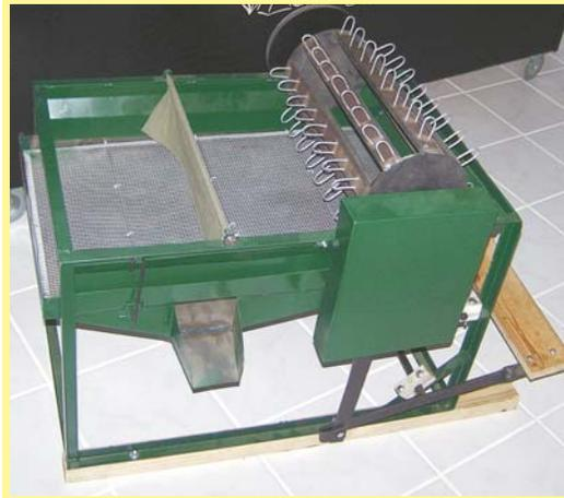
When the treadle is pumped up and down, connecting rods turn the reel and shake the screen.
