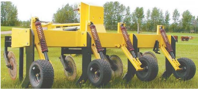
Brandon Janssen's forage "regenerator" cuts through sod, shattering the subsoil and then closing the cut.
