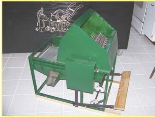
Small-scale thresher consists of a foot treadle, an enclosed threshing reel, and a winnowing screen.
