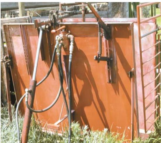
He added a 2-way valve and a hydraulic cylinder, which are powered by a small tractor.
