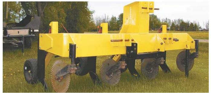
A 16-in. coulters precuts sod layers, and is followed by a shank and coil spring-mounted packer wheel.
