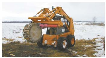
Lewis Legge's quick-tach log splitter mounts perpendicular to skid loader instead of in line with it. As a result, it's coupled closer to the loader and can split bigger logs. A 5-in. dia., 28-in. long hydraulic cylinder bolts onto one side of steel I-beam.
