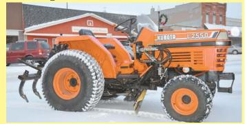
Hydraulic-operated, belly-mount grader is designed to attach to 2 or 4-WD tractors with 45 hp or less. "It lets you grade roads too small or inconvenient for conventional graders on bigger tractors," says inventor Randy Leith.
