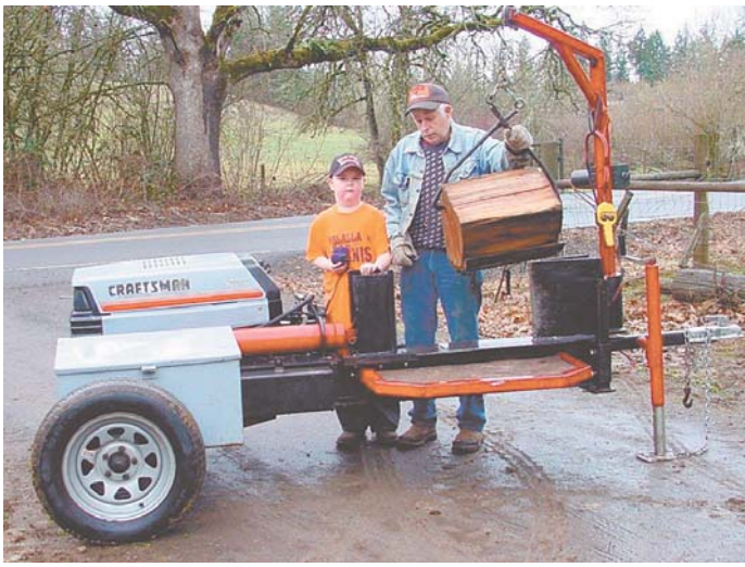
Vance Burns converted a Sears Craftsman riding mower into a handy wood splitter that's complete with a hitch and hoist.
