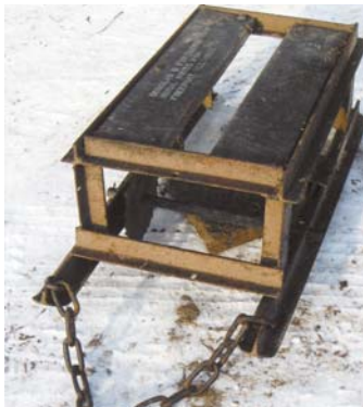
Sod cutter cuts a 12-in. wide, 2-in. thick strip of sod. Photo at right shows unit placed on its side to display saw blades and angled knife.
