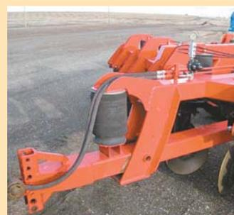
Air bags help disk float over on rough terrain of equal pressure..
