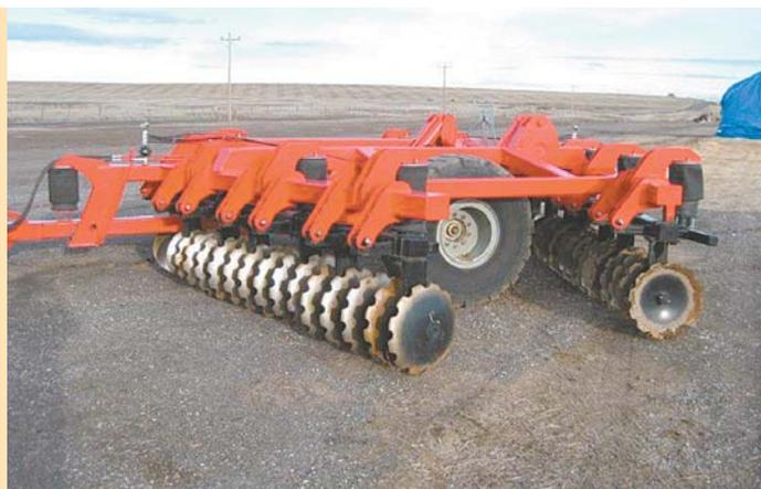
Heavy-duty "Rockzilla" disk uses truck air bags for suspension and to control gang flotation.
