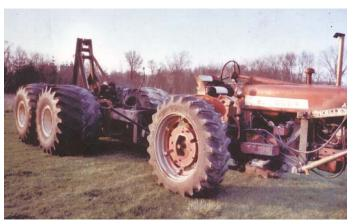
Deane and Dan Sarber built two different "winches on wheels" to pull out stuck machines. Model shown above rides on four big flotation tires off a Big A self-propelled
