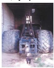
Self-propelled, 4-WD tandem axle winch is designed to lift stuck machine straight up and then pull it out. Cable rides up and over winch on tower at back of machine.
