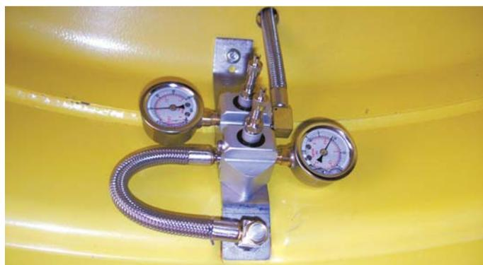
Tire Minders fit single, dual and triple wheels. Photo shows a 2-gauge unit for duals.
