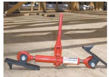
Both ends of the WoodRatchet consist of flat plates fitted with spikes. Ratcheting binder is then used to pull or push stud wall.
