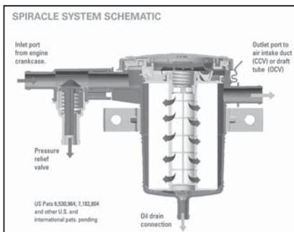
Spiracle filtration unit captures "blow-by" oil from the crankcase and returns it to the engine sump.
