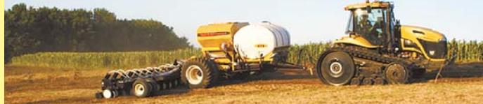
Seed Warrior consists of a 7,500-lb. tank with a 1,250-gal. fertilizer tank.
