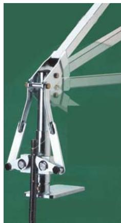
The JackJaw T-Post Extractor works like a ratchet on a jack, except that it grabs the post using a pair of cam-shaped, case hardened steel jaws.
