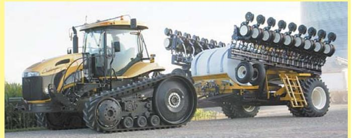
Active hydraulic down pressure provides uniform depth control in varying field conditions.
