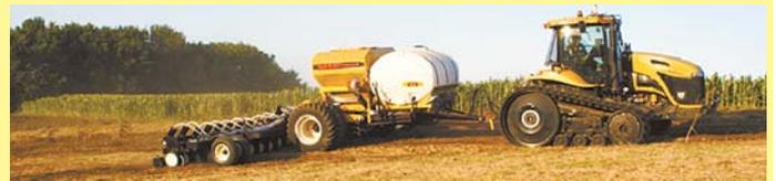
Seed Warrior consists of a 7,500-lb. tank with a 1,250-gal. fertilizer tank.
