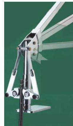
The JackJaw T-Post Extractor works like a ratchet on a jack, except that it grabs the post using a pair of cam-shaped, case hardened steel jaws.
