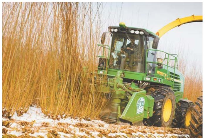
Hydraulically-driven willow header fits a wide range of forage harvesters. It can harvest up to 150 tons per day of chipped wood.
