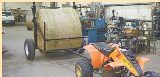
The 2-wheeled bale mover easily converts into a small flatbed trailer and can be used behind a small tractor, car or 4-wheeler.
