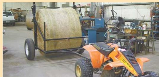
The 2-wheeled bale mover easily converts into a small flatbed trailer and can be used behind a small tractor, car or 4-wheeler.
