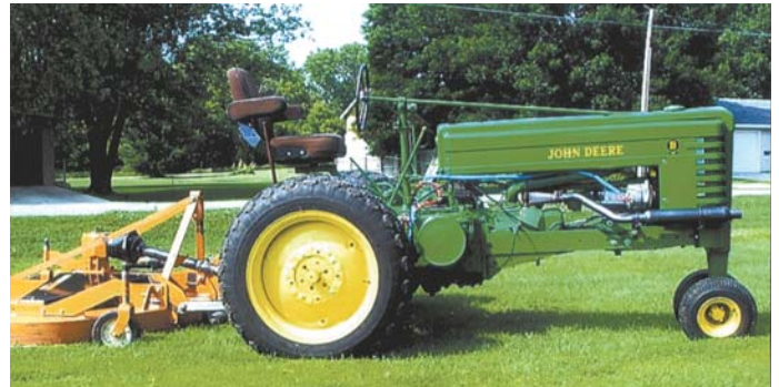
David Owings modified this 1942 Deere "B" tractor to pull an 84-in. Woods rear discharge finish mower.
