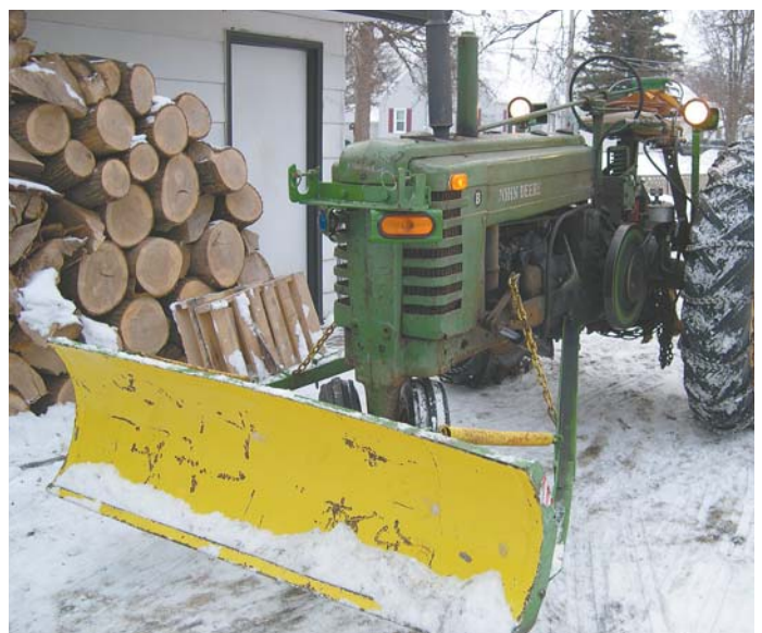
John Bipes mounted a 6-ft. snowplow – which he made by cutting apart an old water tank – on front of his Deere B tractor.
