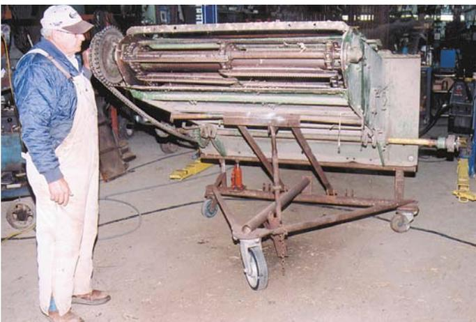
Rolling dolly is fitted with larger caster wheels, which makes it easy to wheel feederhouses around.
