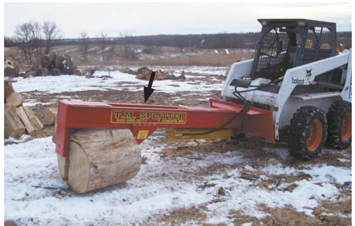
Log splitter is built from two pieces of channel iron mounted back to back, with an 8 by 24-in. “window” in between.
