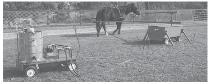
Traveling in a circle, horse drives a gearbox that powers a 600 rpm hydraulic pump which connects to the the ice cream maker.
