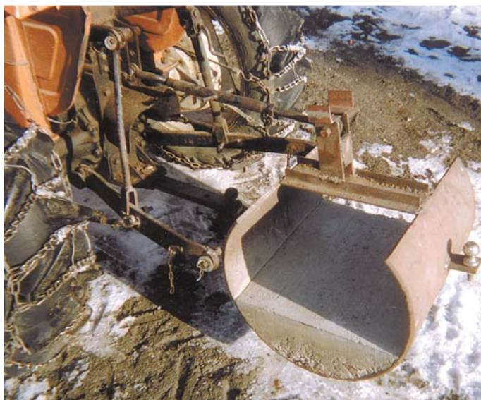
Counterweight is made out of a piece of 24-in. dia., 1/2-in. thick wall pipe. Barrett uses the counterweight when operating a front-mounted boom on his Allis Chalmers tractor.
