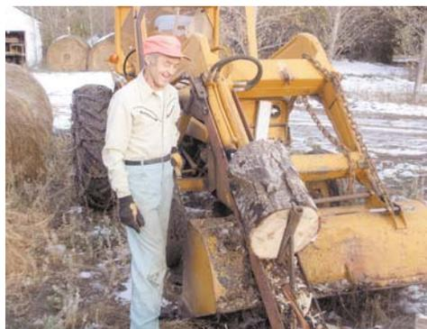
Ken Yettaw built this loader-mounted log splitter for his Ford 9N tractor on-the-cheap, using existing parts and salvaged material.
