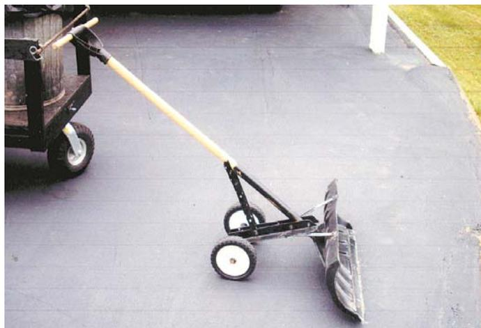
"Wheeled snow pusher" is equipped with a 24-in. wide shovel that rides on a pair of 6-in. rubber wheels.
