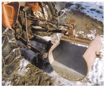
Counterweight is made out of a piece of 24-in. dia., ½-in. thick wall pipe. Barrett uses the counterweight when operating a front-mounted boom on his Allis Chalmers tractor.
