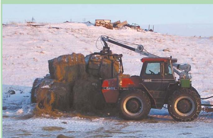
Tractor-mounted boom lets Ruben Auch load round bales into feed wagon without getting off tractor.
