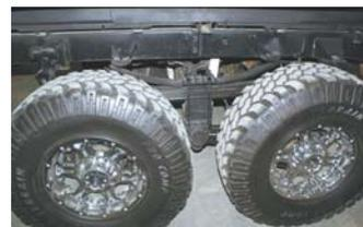
He added an axle in front of pickup's rear axle and installed a military bogie-style suspension, adding three leaves to the existing leaf spring set.
