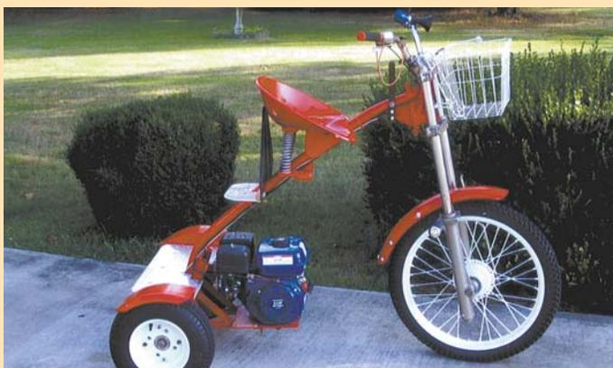
Tricycle rides on a 21-in. high front wheel off a motocross bike and two 8-in. boat trailer rear wheels, which are chain-driven off the engine.
