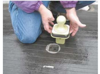
New Shocker Cushion Ball has a poly bump cushion sandwiched between two steel plates to make towing smoother.
