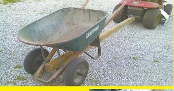
I found an easy way to turn a wheelbarrow into a cart I can tow behind a garden tractor or ATV. I bought an 8-ft. 4 by 4 and laid it over the axle between the front wheels. A couple brackets wrap around the axle and lag-bolt to the 4 by 4 to hold it in place. The wheelbarrow is stock, except for the brackets. A bracket attached to the opposite end pins to the drawbar hitch.
