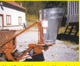
a Herd 3-pt. hitch mounted broadcaster to the front of a Gravely garden tractor. We used a Boston gear #621A speed reducer to get the proper drive shaft direction and speed off the front pto. The seed gate is foot-operated for quick start and stop when broadcasting.
