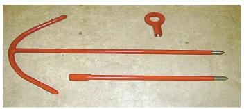
"Plug puller" consists of 5/8-in. cold-rolled rod, bent to an "anchor" shape. After pointed end is poked through plugup, extension and eye bolt are screwed on.
