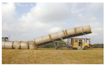
A separate 28 hp Kubota engine provides hydraulic power to clamp, lift and move bales up over top of cab and onto rear bale frame.
