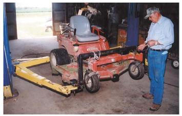
Roger Foster made brackets for his commercial 10,000-lb. rotary hoist to raise and lower his zero-turn riding mower.
