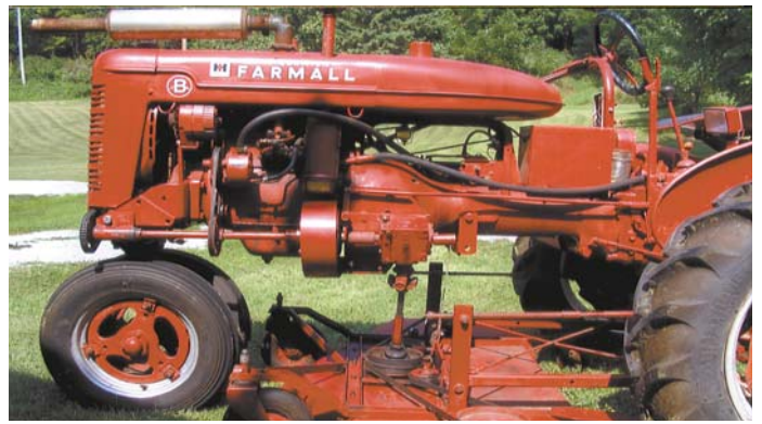
Shaft belt-drives a power steering pump that raises or lowers mower. Shaft also connects to a right angle gearbox that drives mower blades.
