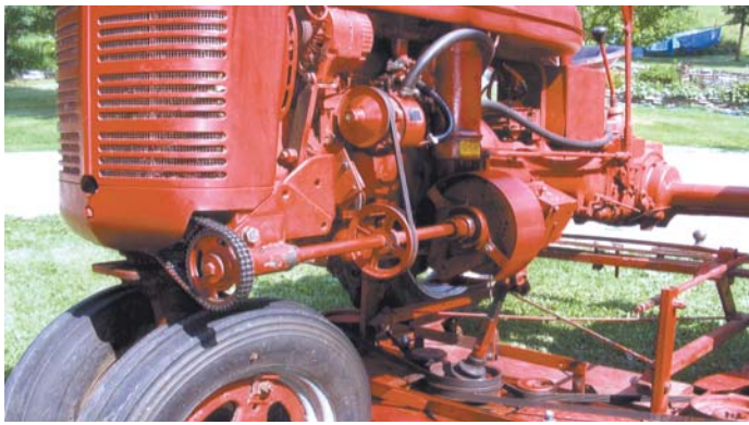
To add live pto to his Farmall, Glen Alstad welded a sprocket to engine's crankshaft. It chain-drives a shaft that runs along side of tractor.
