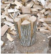
Three 6 to 7-in. "spikes" stick up from top of wood block to hold chunks in place for
