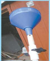
Fertilizer applicator uses a plastic funnel that's screwed to a 1-in. plastic pipe, with a shut-off valve about 16 in. from the top. It holds 1 to 1 1/2 gal. of fertilizer.
