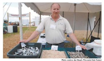
Ag plastic made into pellets with wood fiber and other materials, burns well, says Rabl.
