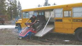
Snowmobile or ATV is driven out the side of bus through a 6-ft. wide, hinged door, which is raised and lowered by an electric boat winch.
