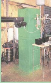
LST pellet stove and hot water boiler burns hay and wood pellets, as well as corn. It eliminates naturally forming clinkers that might smother fire.
