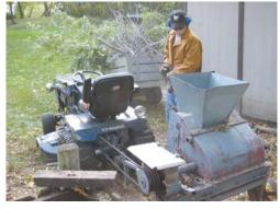
Lloyd Litchy converted an old Gehl stationary silage chopper into a low-cost wood chipper. He uses a garden tractor to beltdrive it.
