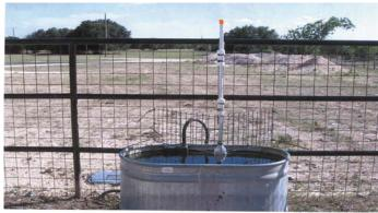
Float attaches to pipe with red cap on top. If the cap drops below the top of fence, Katzenmeyer knows there's something wrong.
