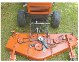
Tractor was originally equipped with a gearboxdriven 42-in. deck, which Mork widened to 48 in. and also converted to belt-drive.
