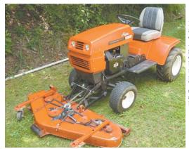
Robert Mork and his son Rob converted a 1977 Ariens S-16 garden tractor equipped with a belly-mounted mower to a frontmount model. The deck is offset so they can more safely mow steep banks.
