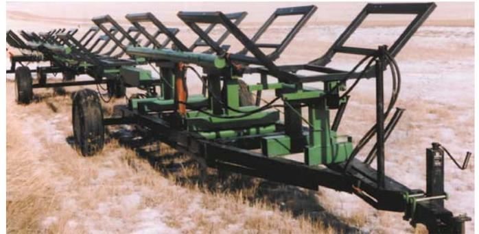
**Cradles on each trailer attach to a single beam that dumps all the bales at once.**
