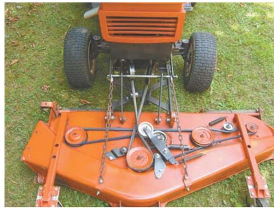
**Tractor was originally equipped with a gearbox-driven 42-in. deck, which Mork widened to 48 in. and also converted to belt-drive.**
