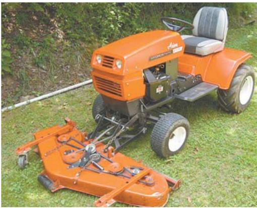
Robert Mork and his son Rob converted a 1977 Ariens S-16 garden tractor equipped with a belly-mounted mower to a front-mount model. The deck is offset so they can more safely mow steep banks.
